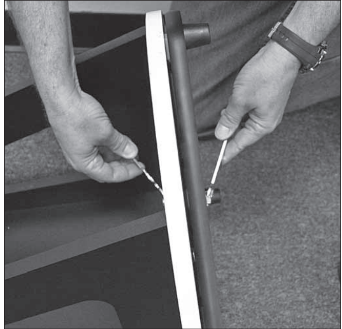
Figure 6. Use the two included open-end wrenches as shown to attach the bottom groundplate to the top groundplate.
