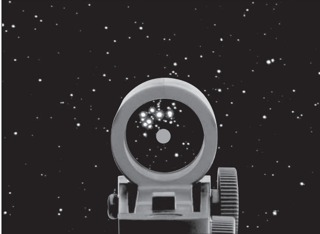
Figure 16. The EZ Finder II superimposes a small red dot (it's not a laser!) on a non-magnified field of view, which helps to center an object in the telescope's field of view.
